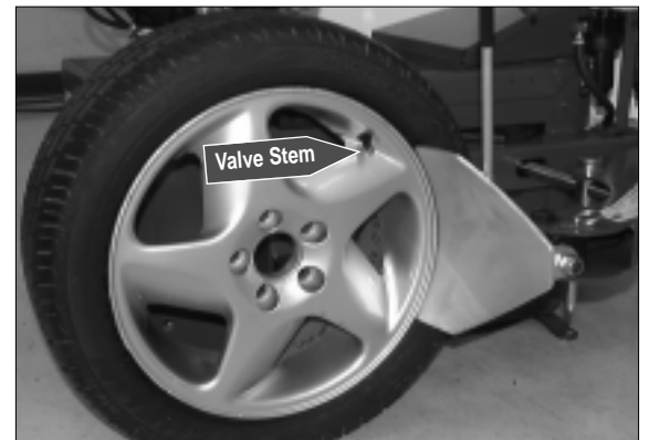
Figure 2 - Position Tire for Bead Loosening
