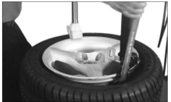
Figure 11 - Rotate Lifting Tool Down for Demount
