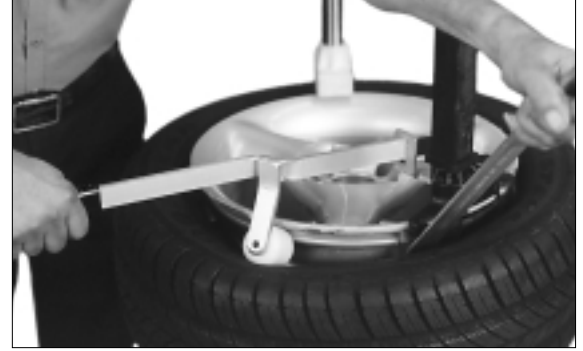
Figure 10 - Insert Bead Lifting Tool
