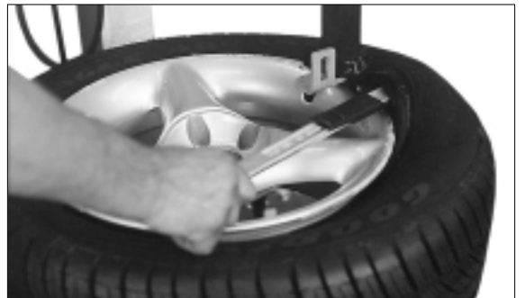
Figure 12 - Holding Lifting Tool in Place and Rotate Wheel
