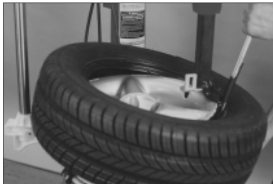
Figure 14 - Helper Holding the Lower Bead in Drop Center
