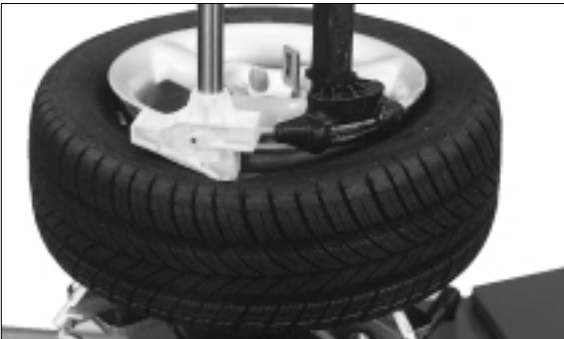
Figure 7 - Helper Foot Depressing Sidewall of Tire
