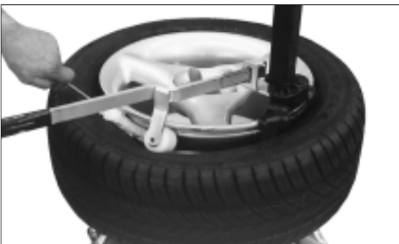
Figure 8 - Lubricate Upper Bead
