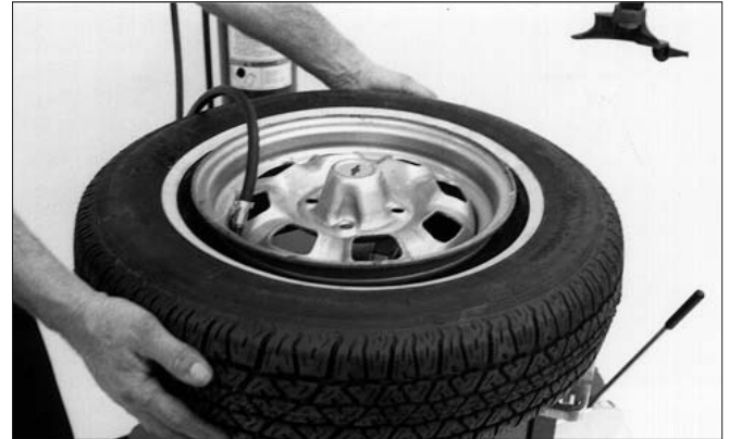
Figure 25 - Lift Tire Upwards for Bead Sealing
