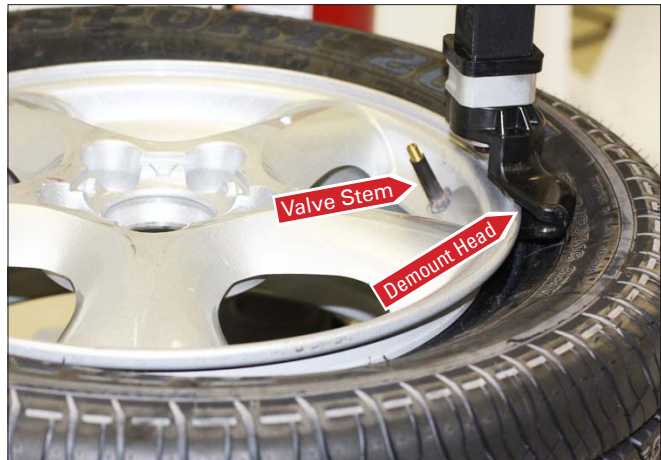
Figure 17 - Position Valve Stem Behind Demount Tool Tail
