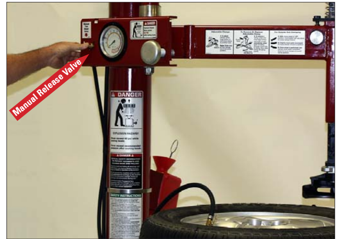
Figure 27 - Location of Manual Release Valve
