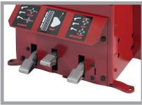
Provides precise control over every step of the changing process. The pedals are ideally placed for fluid technician movements while mounting and demounting tires.
