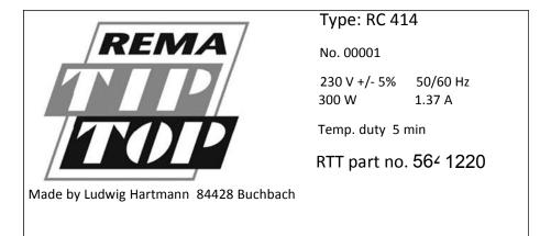
The data shown here is given as an example and will vary depending upon the rated voltage and model of the tyre regroover.
