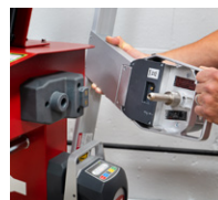
Side supports house and recharge measuring head batteries
