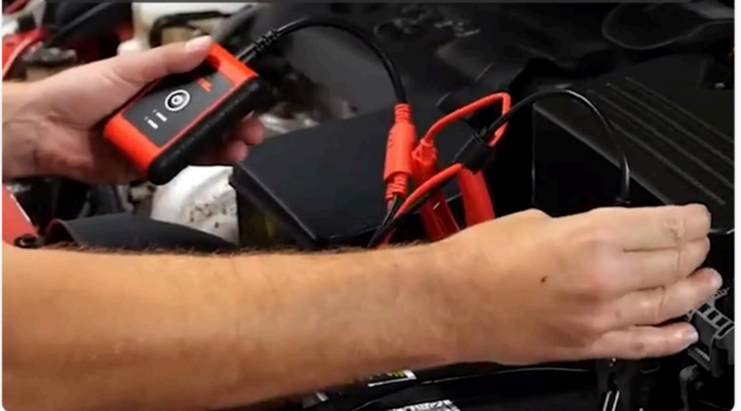
Figure 4.1: Performing an in-vehicle battery test with the BT506.
