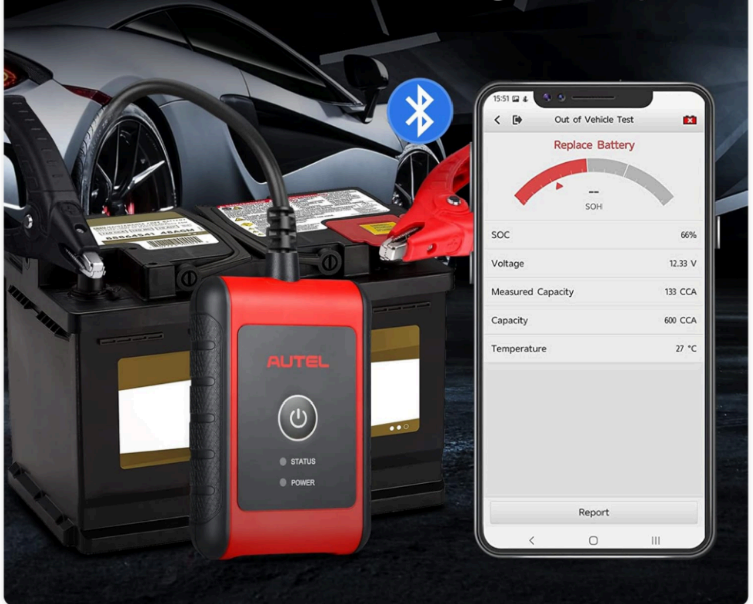
Figure 4.2: Performing an out-of-vehicle battery test with results shown on the connected smartphone.
