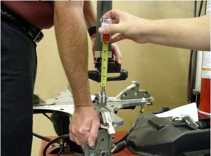
3. Subtract step 1 distance from step 2 distance. If distance is greater than 3/8-inch then machine is not compatible.
