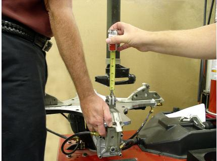
2. Now, pull up on mount/demount head while pushing down on table top. Record distance - top of clamp to bottom of mount/demount head.
