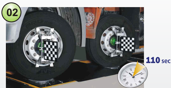
One shot Caster swing of twin steer axles
