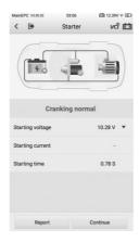
Figure 6-11 Starter Test Result Screen
