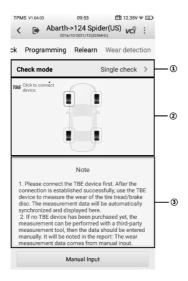
Figure 4-29 Wear Detection Screen
