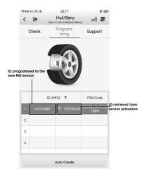
Figure 7-5 Programming Screen via OEM Part No.
