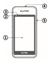
Figure 2-1 MaxiTPMS Tablet Front View
