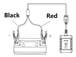
Figure 6-2 Connecting to a Battery
