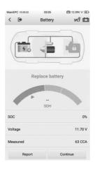
Figure 6-8 Battery Result Screen
