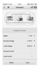
Figure 6-12 Generator Test Result Screen
