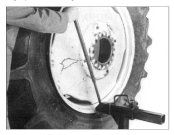
**2.** With the spade tool inserted between the rim and the outer bead, on the right of the combo tool, pry the bead out over the rim edge.
