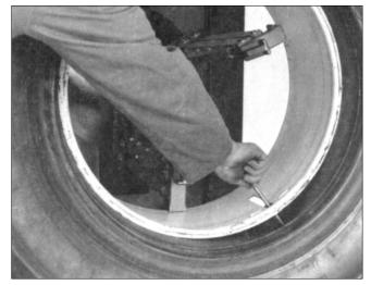
**5.** Rotate the wheel and slowly advance the disc to push the tire about half way off the wheel. Push the valve stem inside the wheel, then finish pushing the tire off the wheel.
