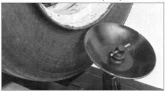
**2.** Position the bead loosening disc in one of the square holes in the carriage closest to the outer edge of the tire.
