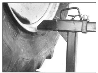
**1.** Advance the combo tool close to the rim, with the finger past the rim edge.
