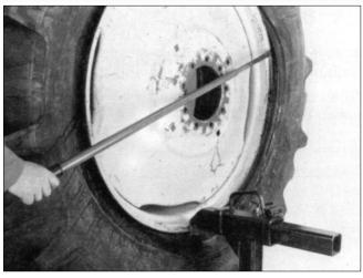
**3.** Rotate the wheel counterclockwise while maintaining pressure on the spade tool until the outer bead is demounted. Push the valve stem inside the rim and pull the inner tube out of the tire.
