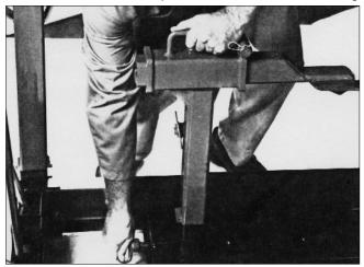
3. Install combo tool retaining pin into carriage.
