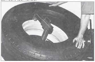
**5.** Mount Bottom Bead: Depress front of either foot pedal, thus rotating the tool clockwise. Hold down on the tire until the tool begins to mount the bottom bead. Make sure the bead goes into drop center behind the tool head.
