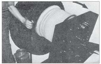
**8.** Remove Tire: After demounting the bottom bead, lower table to free rim from tire.
