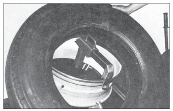
**4.** <u>Position Tire:</u> Lower table to a comfortable angle and rotate tool to approximately the 7 o'clock position. Lean tire over the rim and hook lower bead on mount/demount tool handle.
