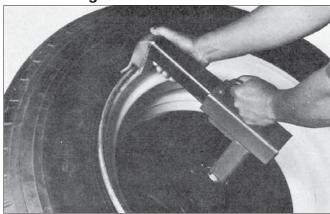
**1.** <u>Install Mount/demount Tool:</u> Insert mount/demount tool in square drive socket and position tool head on the rim flange. Rotate the tool head to approximately a 12 o'clock position by depressing either foot pedal.
