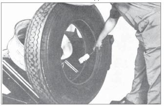
**3.** <u>Lubricate Tire Beads:</u> After inspecting tire thoroughly, lubricate both beads inside and out with an approved lubricant.
