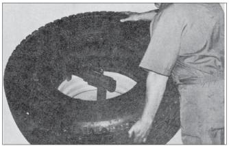
**1.** Mount Bottom Bead: With the table at a comfortable angle, mount the bottom bead in the usual manner. It may be necessary to lift the bottom bead into drop center as the mount/demount tool rotates.
