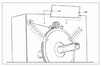
**6.** Lubricate Ring Gear: To gain access to the pinion and ring gear, remove the COATS name plate located on the working table. With a small brush or grease gun, apply AGMA #1 or #2 grease liberally on the ring gear teeth.
