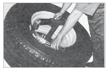
**4.** Lubricate tire beads and rim flange thoroughly: It may be easier to lubricate the top bead by letting the mount/demount tool push down on the bead and then rotating the tool with the lube swab following the tool. Demount the top bead in the usual manner). See section one.
