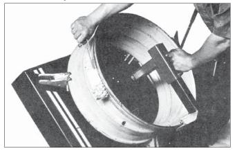
**2.** <u>Lubricate Rim:</u> After inspecting rim, thoroughly lubricate both bead seats with approved tire lubricant.
