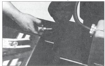
**1.** Oil Level Check: Remove filler cap and check oil level on dip stick. Fill to proper level as needed. Use hydraulic oil only.
