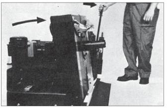
**1.** Raise working table: Raise working table to almost vertical position by pulling back on the control handle. Open clamps by twisting the control handle counterclockwise.
