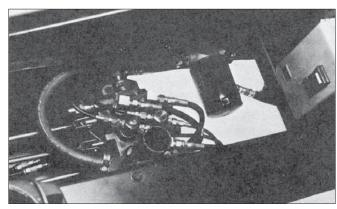
**7.** Oil Filter Change: Disconnect electrical power. Remove cover panel and place a shallow pan under oil filter. Remove oil filter with standard auto oil filter grip or wrench. Replace with service part #8120222.
