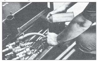
**3.** Oil Air Lines: Disconnect air supply at rear of machine. Remove cover plate and disconnect quick coupler connection between air valve and cylinder. Use fair amount of spray lubricant.
