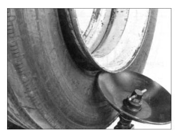
**3.** Rotate the tire. While the tire is rotating, slowly advance the bead loosening disc to contact the tire bead. Adjust the chuck up or down so the disc is close to the rim.
