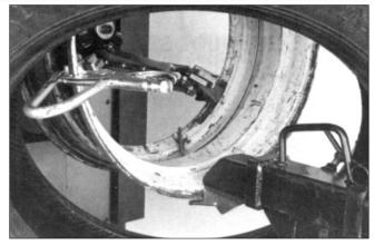
**3.** Position the combo tool near the edge of the rim as shown. DO NOT CONTACT THE RIM.
