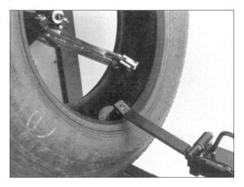
**1.** With the tire completely demounted and the rim removed from the clamps, hook the inner bead over the clamps and the roller tool over the outer bead. Move the tool away from the inner bead to gain access to the inside of the tire.
