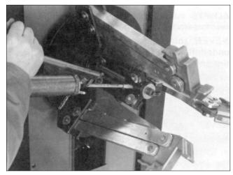
**1.** Using a grease gun and chassis grease, lubricate chuck hub bushing once every month.
