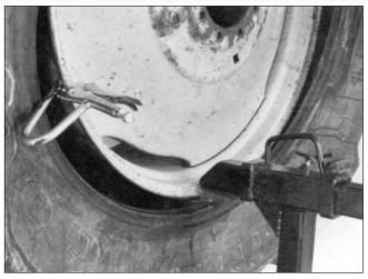
**3.** Move the combo tool into position near the edge of the rim.
