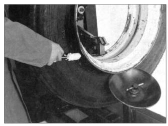
**5.** While the tire is still rotating, apply a liberal amount of tire lubricant to the tire bead and the rim.
