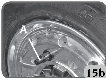
The pressure should be reduced for weak or particularly thin rims; for thick rims that are difficult to demount, it is recommended to adjust pressure to the maximum level. Adjust the turntable opening by means of the "closing/opening" command (A fig.?), according to the type of rim to be locked (see the examples in fig.16).
