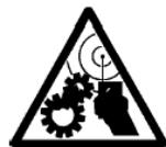
Machine with remote controlled movements.
