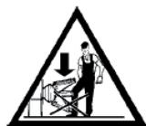
During the descent of the turntable spindle (both with a wheel mounted and with the turntable open), keep at a safe distance to avoid any possible risk of getting crushed.
