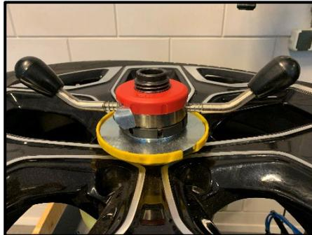
**STEP 4** UNSCREW THE QUICK NUT AND REMOVE PLASTIC CONE COVER HOLDING THE DUAL METAL CONES.
