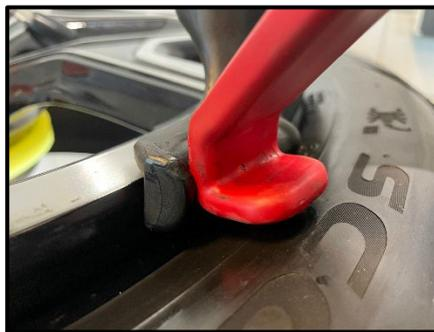
**STEP 23** DEPENDING ON THE TIRE COMPLEXITY, USE THE HELPER ARM (2) AND ITS PRESS BLOCK TO GENTLY PRESS THE TIRE BEAD ON THE OPPOSITE SIDE. THIS TO MAKE SURE THAT THE BEAD IS IN THE DROP CENTER TO ENSURE SUFFICIENT SPACE WHILE DEMOUNTING WITH THE IN-CONTROL HOOK AND (DE)MOUNT HEAD. ELUBE TIRE SPRAY PLAYS A CRUCIAL ROLE DURING MOUNTING AND DEMOUNTING.
