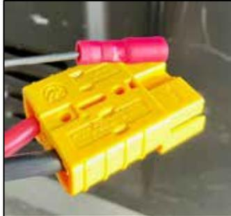
The second Anderson connector comes separately and should be handed over to the installer.
