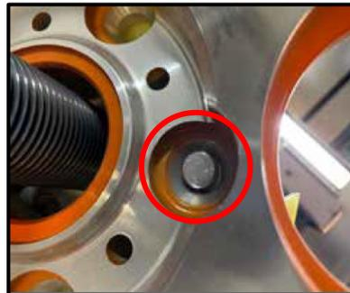
**STEP 4** CHECK IF CENTER HOLE OF THE RIM IS LINED UP WITH THE CENTER POST SPINDLE. THEN PRESS AND HOLD THE **RIGHT FOOT PEDAL** TO ELEVATE THE CENTER POST SPINDLE TO ITS MAX HEIGHT.
