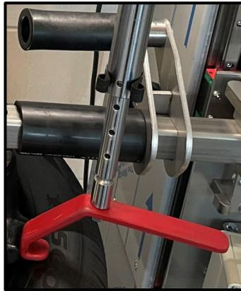
**STEP 20** RAISE THE VERTICAL TOOL SELECTOR UNTIL THE (DE)MOUNT HEAD ARM CAN MOVE FREELY OVER THE TIRE. MOVE THE ARM TO ITS LOCKING POSITION.
