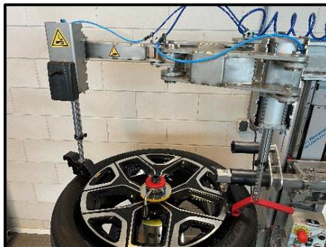
**STEP 24** LOWER THE HOOK, BY OPERATING THE PNEUMATIC CYLINDER, UNTIL IT GRABS THE TIRE BEAD. DURING THE PROCESS (BOTH UPWARDS AND DOWNWARDS) IT'S CRUCIAL TO GUIDE THE HOOK BY HOLDING THE GRIP.
