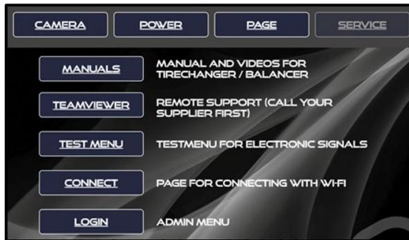
The test menu tab helps to quickly identify a possible connection problem between components.
