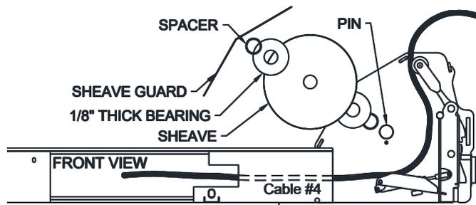
Fig 8 – Cable #4 Routing
