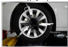
Tire gripping design eliminates the risk of wheel damage.
