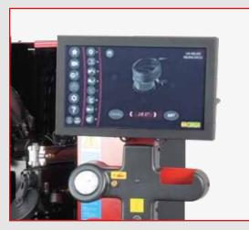
Master Force allows to use the tyre changer through the **automatic work cycle**. The management software improvement, thanks to Corghi's experience, is aimed at **preserving rims and tyres**.
