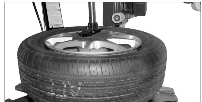
Figure 7 - Robo Arm Aids Clamping
