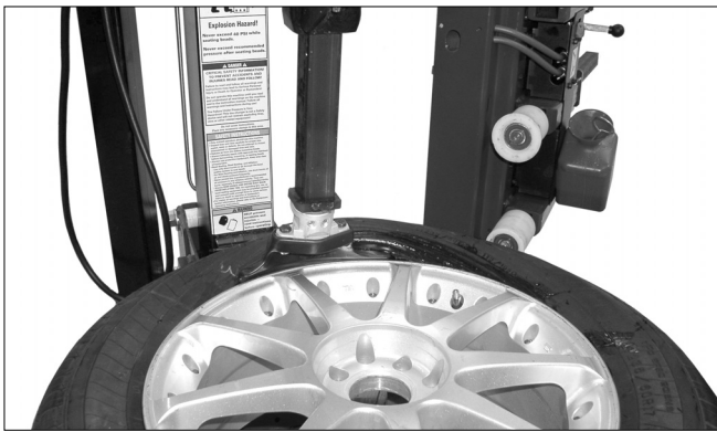
Figure 12 - Demount Upper Bead
