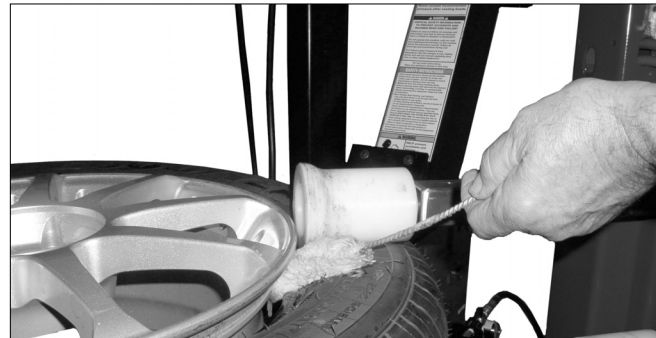
Figure 10 - Apply Rubber Lubricant to the Beads
