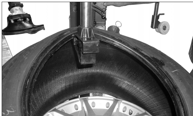
Figure 13 - Lift the Tire for Lower Bead Removal
