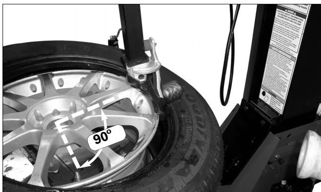
Figure 20 - Position Valve Stem 90° Ahead of Duckhead
