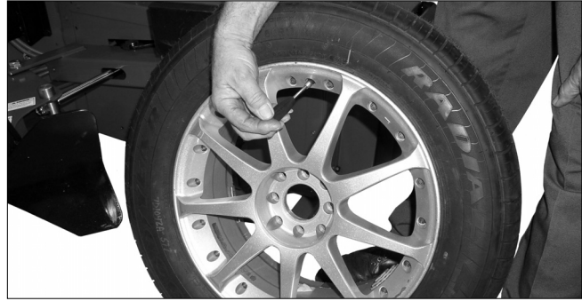
Figure 1 - Remove Valve Core to Deflate Tire
