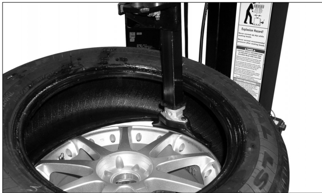
Figure 19 - Mounting Lower Bead
