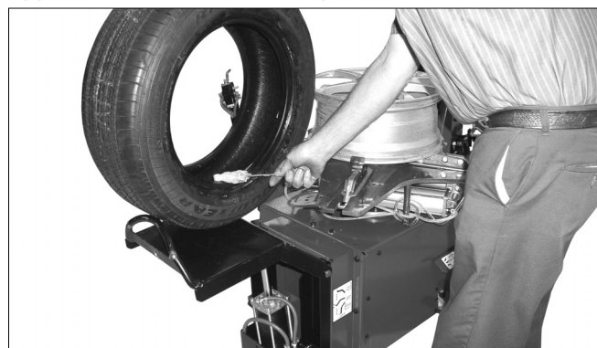
Figure 17 - Lubricate Tire Beads Liberally
