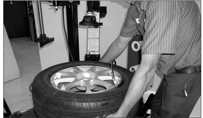
Figure 23 - Lift Tire Upwards for Bead Sealing
