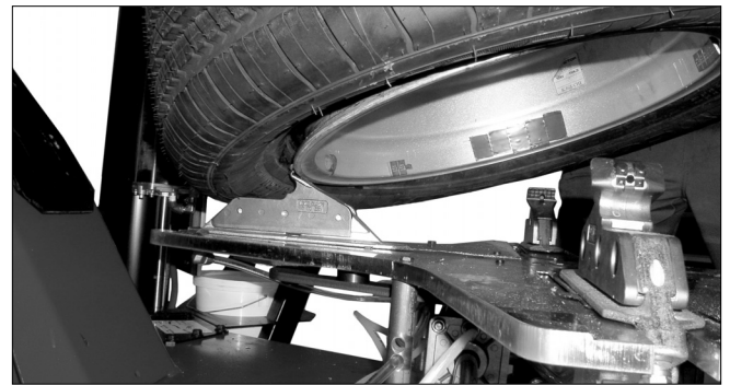
Figure 6 - Clamp Outside on Mag Wheels
