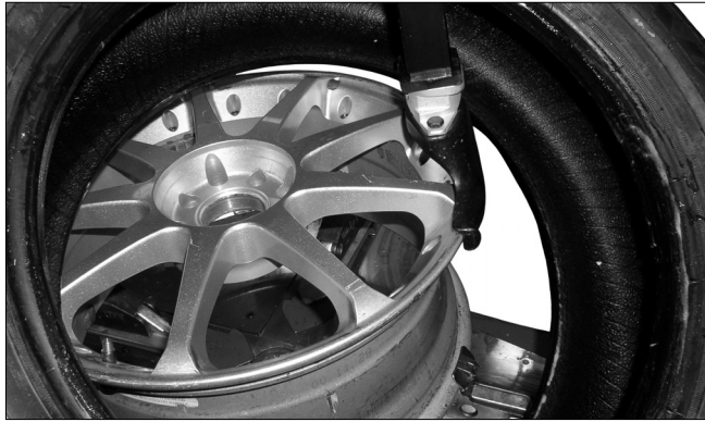
Figure 18 - Position Tire Against Duckhead®
