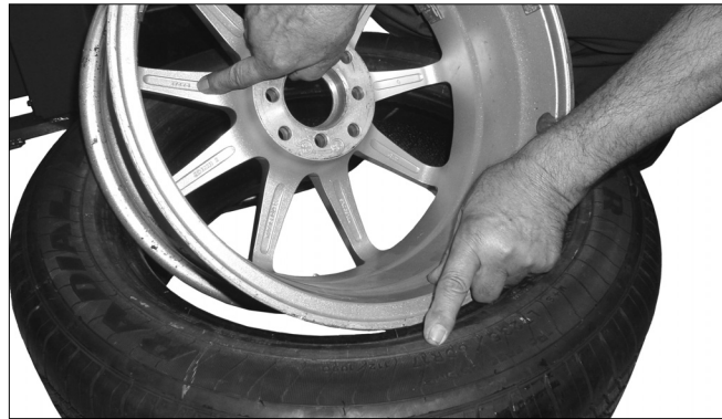
Figure 15 - Verify Size Match Between Tire and Wheel
