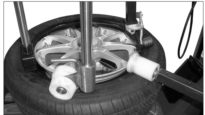
Fig 22 - Use RoboRoller (if equipped) To Hold Tire In Rim Drop Center
