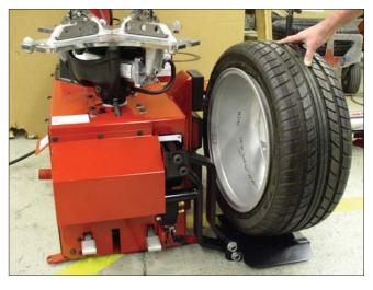
**2.** With wheel assembly on wheel lift. Keep wheel vertical and push foot pedal down to raise wheel up.
