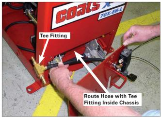
**8.** Install the tee fitting, from the new pedal bracket assembly, into the just cut 3/8-inch hose and secure using hose clamps.
