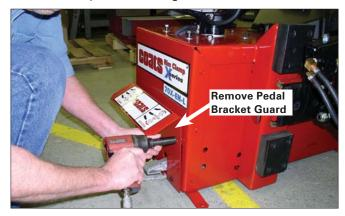
**5.** Remove the machine's side panel using a speed handle or drill and 3/8-inch socket.
