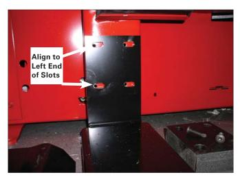
**3.** Now reassemble the lower bead loosener pad over the anti-tip bracket, as shown.
