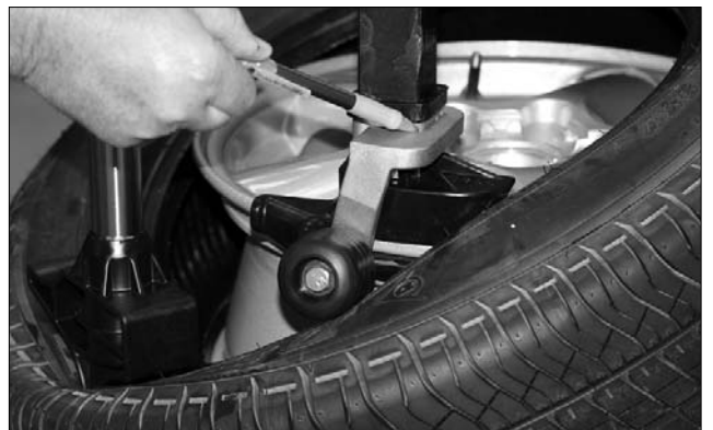
Figure 4 - Duckhead Roller Properly Mounted On Bracket
