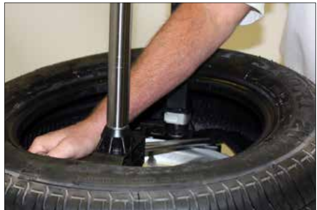
Figure 19 - Guide Lower Bead Over Knob On Demount Tool
