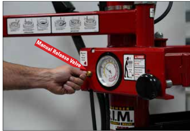
Figure 30 - Location of Manual Release Valve
