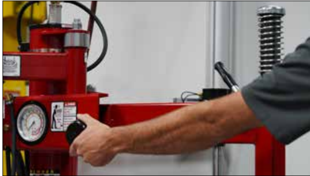
Figure 12 - Adjust Swing Arm to Position Tool
