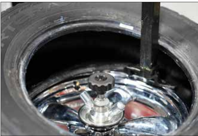
Figure 24 - Mounting Lower Bead
