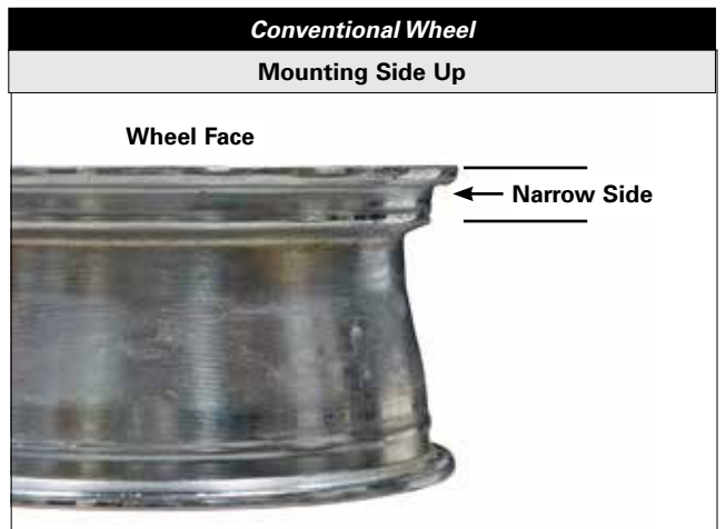
Figure 7a - Mounting Side Up, Conventional Wheel
