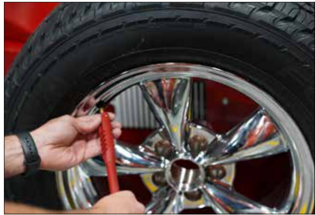
Figure 1 - Remove Valve Core to Deflate Tire
