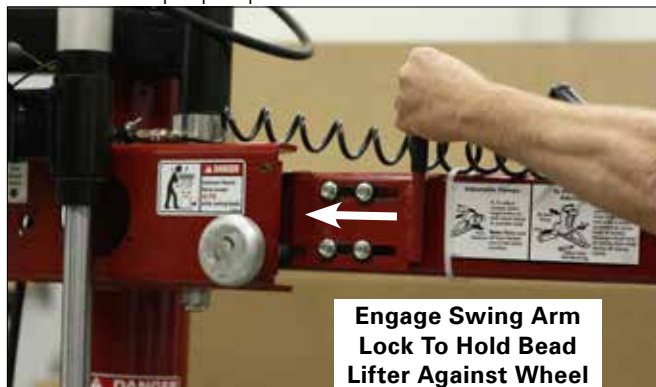
Figure 48 - Lock Swing Arm In Position
