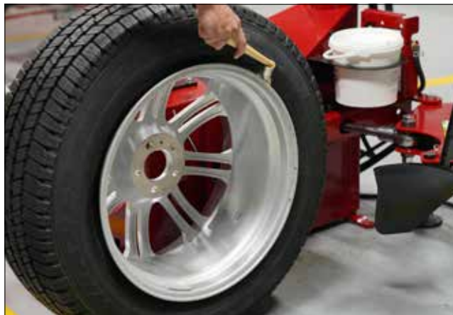
Figure 5 - Apply Rubber Lubricant to Tire Beads
