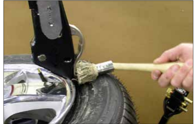
Figure 49 - Apply lubricant to Bead Lifter Tool Hook
