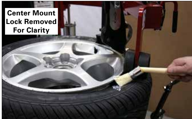
Figure 56 - Use Robo-Roller When Applying Lubricant to Tire Bead
