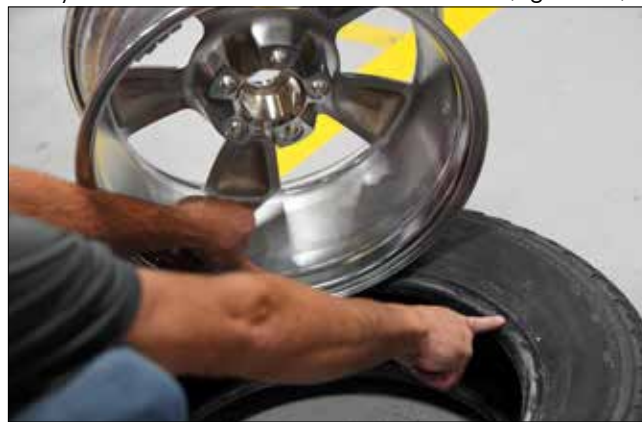
Figure 20 - Verify Size Match Between Tire and Wheel
