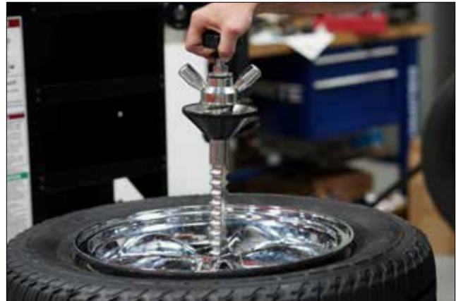
Figure 9 - Place Center Mount Lock through Wheel Center
