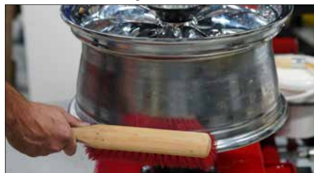
Figure 21 - Inspect and Clean the Wheel
