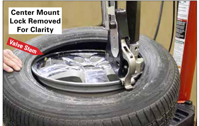
Figure 59 - Position Valve Stem In Front Of Bead Lock
