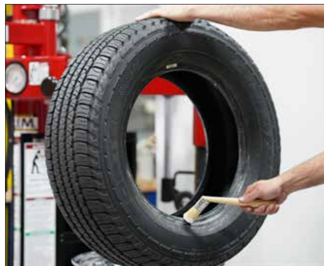
Figure 22 - Lubricate Tire Beads Liberally
