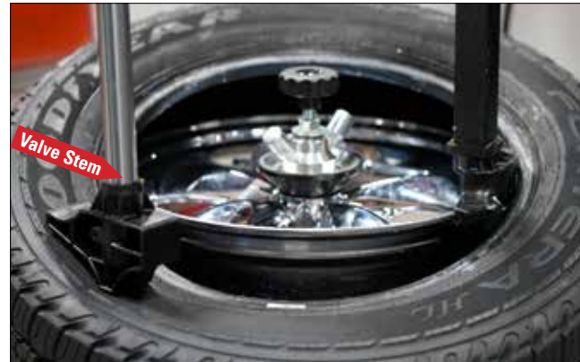
Fig 25 - Use Robo-Arm Helper Device To Hold Tire In Rim Drop Center
