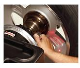
Laser Guided Operation<sup>™</sup> Pinpoints accurate Tape-A-Weight placements.
