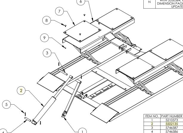
DESCRIPTION QTY. REV LR-60/60P SAFETY BAR ASSEMBLY D CYLINDER ASSEMBLY Ø3.0 X 18 Ε **UPPER HINGE PIN** В DLR-6/LR-60 LOWER CYLINDER PIN В 5 5505400 COTTER PIN Ø6 x 50mm 4 6 5600526 LR-60 LIFT WELDMENT Κ 7 5715048 DLR-6, LR-60 RAMP BOLT-ON RUBBER PAD 4 Α 8 5530364 ELEVATOR BOLT M6 x 1.0 x 25 16 9 5535357 NUT M6 x 1.0 NL 16 В
