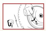
2. Turn T-Handle 1/4 turn to hook valve stem and pull out.
