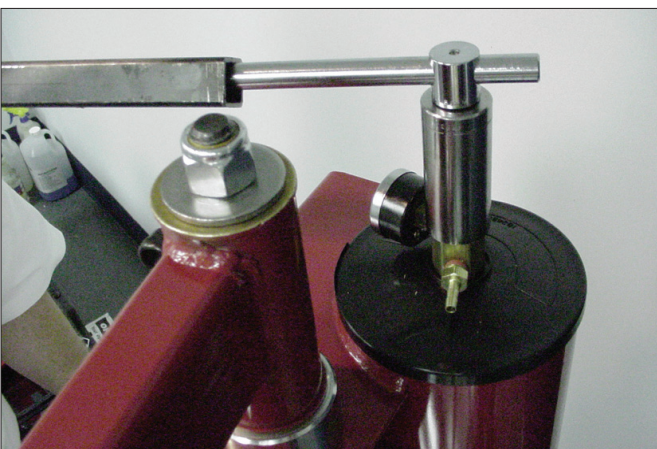
Figure 3 - Install manifold, safety valve and barbed fitting.
