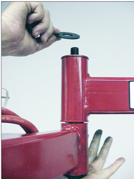
Figure 7 - Hold swing arm in position to install nut to bolt
