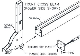
Fig 18 - Front CrossBeam Installation
