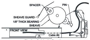
Fig 8 - Cable #4 Routing
