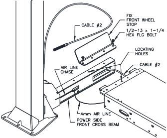
Fig 17 - Front CrossBeam Installation
