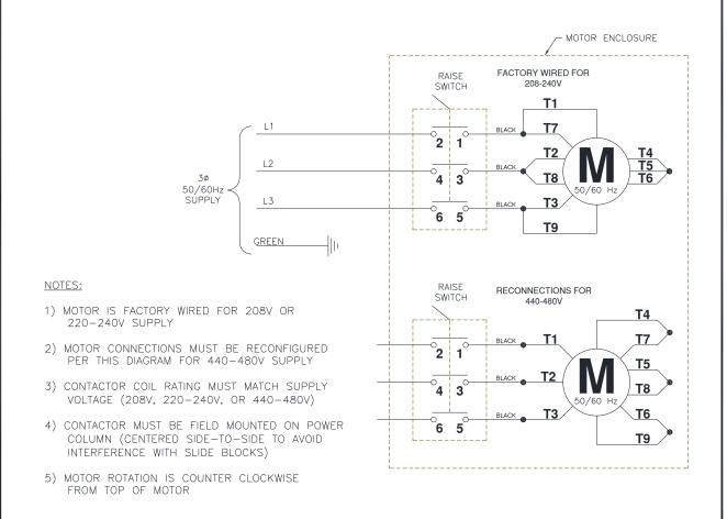
Fig 22 - Electrical Wiring Diagram
