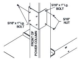
Fig 21a - Power Unit Bracket
