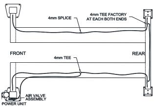
Fig 23 - Lock Release Air Line Routing
