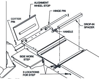
Fig 27 – Alignment Wheel Stop & Turn Plate Installation
