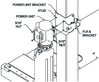
Fig 21b – Power Unit Bracket & Power Unit Mounting
