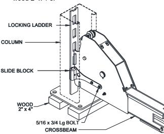
Fig 15 - Slide Block Installation
