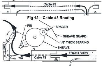
Fig 13 – Cable #3 Routing NOTE: Look through the idler end of the crossbeam and ensure that cable #1 and #3 have not crossed. *Cable* #3 should be above Cable #1.
