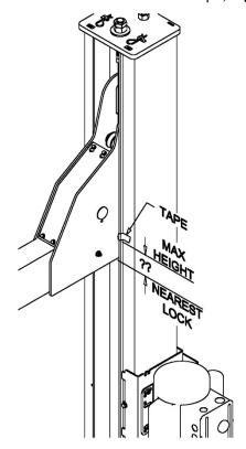
Fig 25 - Lock Clearance Measurement
