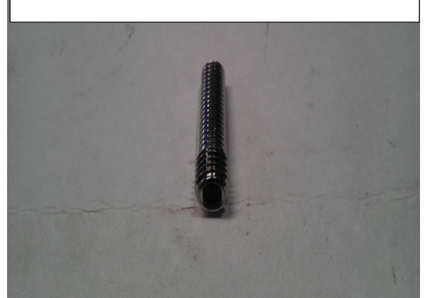
I Model Universal trailing insert roller pin; used to hold Plastic in place; Part#5327727
