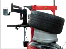
Demounting lower bead
