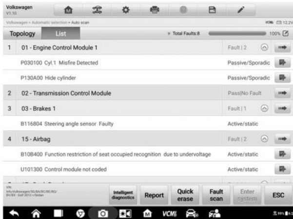
Figure 5-7 Sample Fault Scan on List Screen
