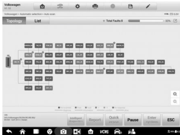
Figure 5-6 Sample Fault Scan on Topology Screen
