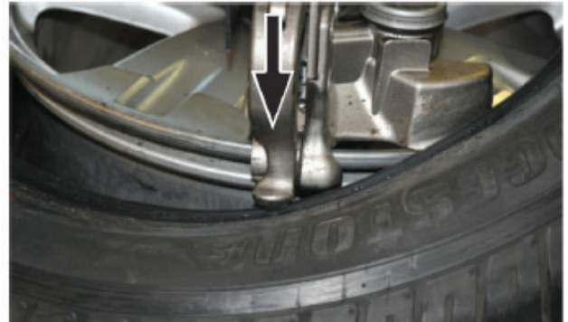
fig. 2 Bead correctly positioned over the left side of the mounting tool and under it on its right side, thus it can be slightly lowered for easy tire mounting.
