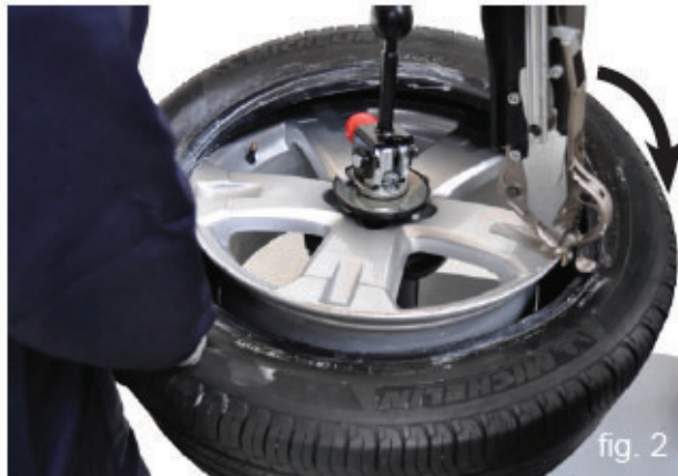
fig. 3 Press the pedal 2 to rotate the wheel clockwise, contemporarily press the tire manually from "5 o'clock" position to force the upper bead at drop-centre position. Keep it pressed while rotating up to "8 o'clock" position to complete the upper bead mounting (fig. 2).
