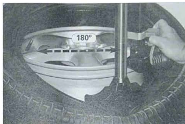
Figure 3 - Position Valve Stem 180° Ahead of Duckhead
