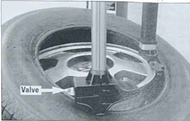
Figure 6 - Use RoboArm To Hold Tire In Rim Drop Center
