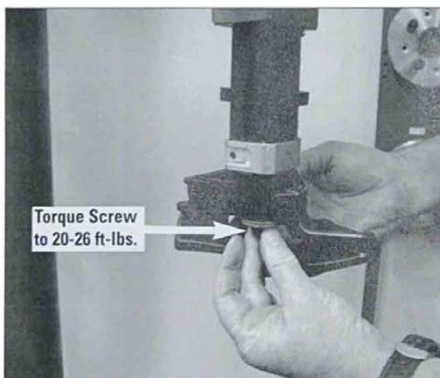
Figure 2 - Reinstall Duckhead
