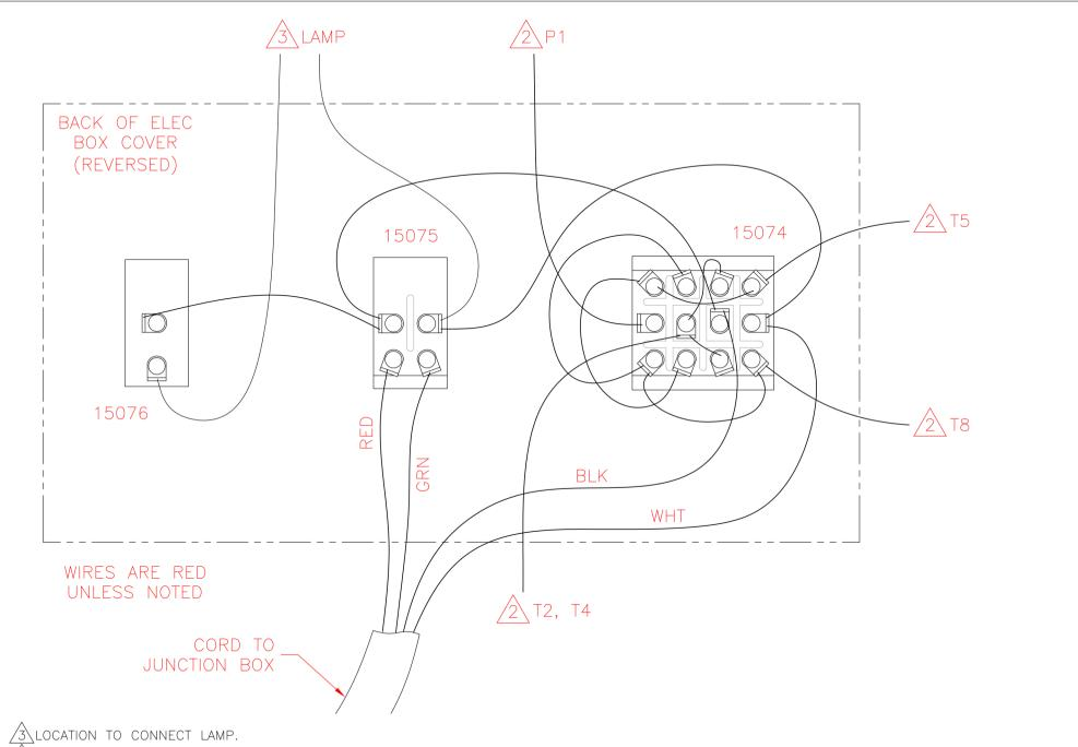
2\WIRES P1, T2, T4, T5 & T8 REFER TO A LEESON MOTOR SOURCE. THE SAME LEADS CAN BE USED ON A MARATHON MOTOR SOURCE.
