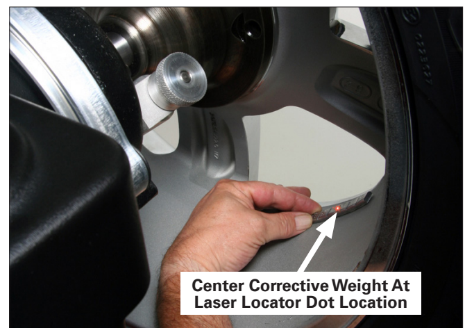
Figure 17 - Centering Corrective Hidden Weight at Laser Dot Location.
