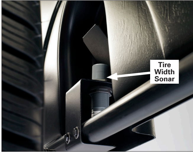
Figure 18 - Tire Width Sonar Located Inside Hood
