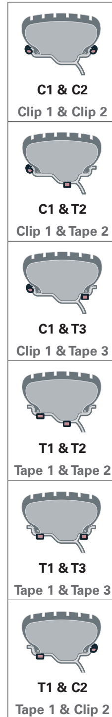
Figure 32 - Dynamic Balance Weight Locations
