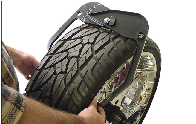
Figure 31 - Caliper Placement On Wheel
